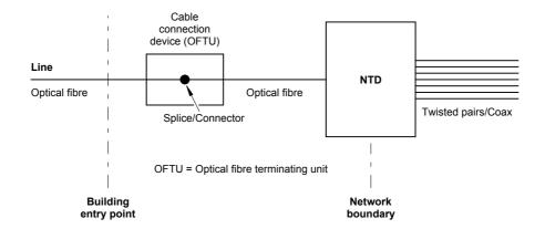
Note: An optical fibre connection device is not an MDF, even if it contains crossconnections, because an MDF only provides for electrical (as distinct from optical) termination of lead-in cabling.
