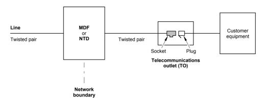
Note: In the above case, the installation satisfies section 22 (4)(a)(i) or section 22 (4)(a)(ii) of the Act, as applicable, so section 22 (4)(a)(iii) of the Act does not apply (refer to Figure J.1). The network boundary is at the MDF or NTD, as applicable.
