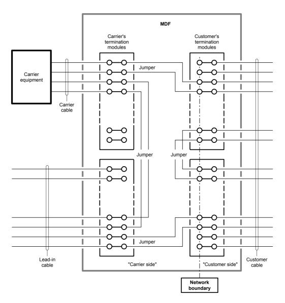
Note 1: The 'side of frame nearest to the end-user' is the 'customer side' of the MDF, i.e. the termination modules and other hardware provided by the customer's cabling provider. Lead-in termination modules and other hardware provided by the carrier are on the 'carrier side' of the MDF.
