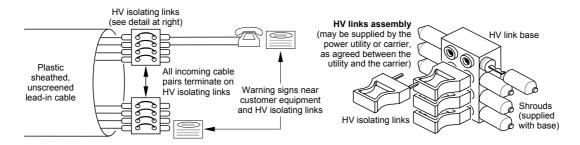
Note 1: The diagram above shows a simple installation without an MDF. Where an MDF is installed, the HV isolating links are installed between the building entry point and the MDF. The HV isolating links should be removed prior to performing any cabling work or customer equipment repairs.
