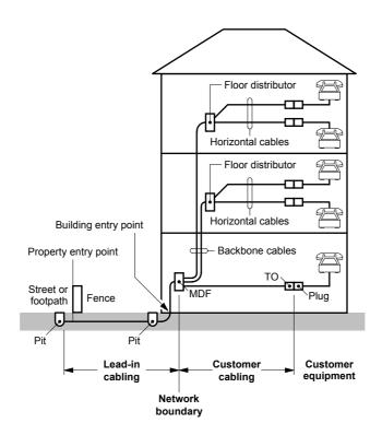
Note: In the above case, the installation satisfies section 22 (4)(a)(i) of the Act (refer to Figure J.1). The MDF is the network boundary for all lines that are connected to that MDF.
