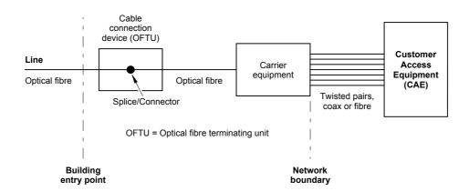
Note 1: In the above case, the installation does not satisfy section 22 (4)(a) or section 22 (4)(b) of the Act, so section 22 (4)(c) applies (refer to Figure J.1). The network boundary is the outer surface of the fixed facility nearest to the end-user. In practical terms, this will be the terminal blocks or connectors on the 'customer side' of the carrier equipment.
