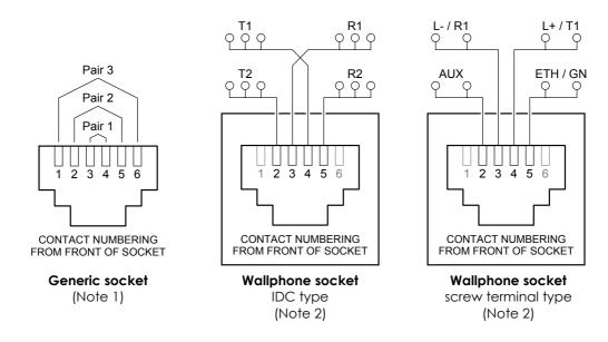
Note 1: The outer contact springs (1 and 6) are not fitted on some 6P modular sockets.
