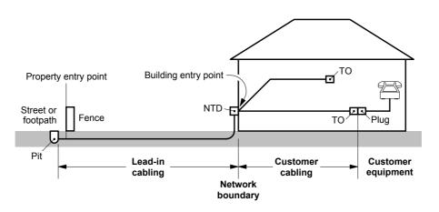
Note 1: In the above case, the installation does not satisfy section 22 (4)(a)(i) of the Act but satisfies section 22 (4)(a)(ii) (refer to Figure J.1). Therefore, the NTD is the network boundary for all lines that are connected to that NTD.
