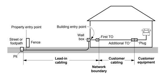
Note 1: In the above case, the installation does not satisfy section 22 (4)(a)(i) or section 22 (4)(a)(ii) of the Act but satisfies section 22 (4)(a)(iii) (refer to Figure J.1). Therefore, the first TO is the network boundary for all lines that are connected to that TO.
