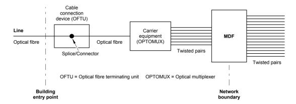
Note: An optical fibre connection device is not an MDF, even if it contains crossconnections, because an MDF only provides for electrical (as distinct from optical) termination of lead-in cabling.
