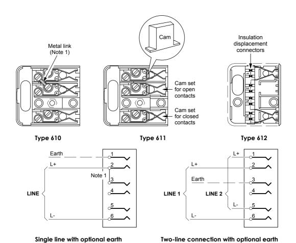
Note 1: A metal link or strap is required between terminals 2 and 3 with older customer equipment to provide a circuit for the ringer (bell).
