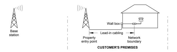
Note: In the above case, while radio is used to supply the service to the customer's premises, the final method of supply is by means of a line (cable) that enters the building. Therefore, section 22 (4)(a) of the Act applies and the network boundary will be at the MDF, NTD or first TO, as applicable (refer to Figure J.1).
