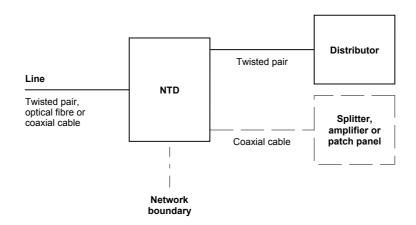
Note: In the above case, the location of the network boundary hinges on the definition of 'Main Distribution Frame (MDF)' in this Standard. In accordance with the MDF definition, the distributor is not an MDF because it does not terminate a carrier's lead-in cabling (the lead-in cabling is terminated on the NTD). Therefore, the installation does not satisfy section 22 (4)(a)(i) of the Act but satisfies section 22 (4)(a)(ii) and the network boundary is at the NTD (refer to Figure J.1).
