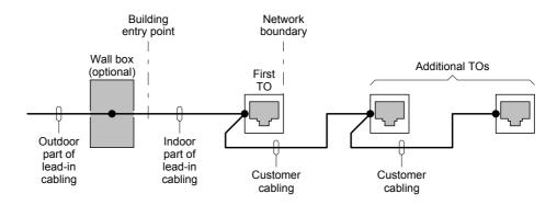
Note 1: In the above case, the installation does not satisfy section 22 (4)(a)(i) or section 22 (4)(a)(ii) of the Act but satisfies section 22 (4)(a)(iii) (refer to Figure J.1). Therefore, the first TO connected to a cable or pair is the network boundary for that cable/pair.
